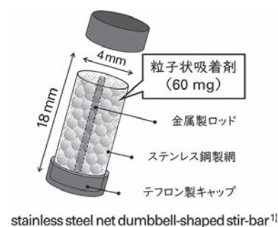
stainless steel net dumbbell-shaped stir-bar 1)
